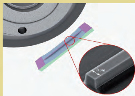
Precision dice & polish LiNbO 3 ridge - Dicing -
